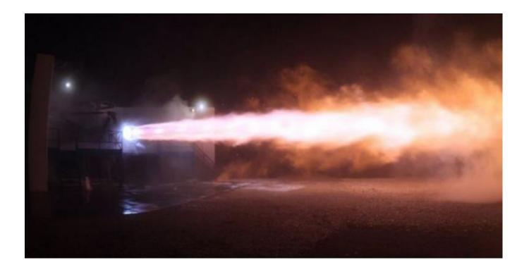
Private firm SpaceX has carried out its first test of the Raptor rocket engine, designed to send humans to Mars.
