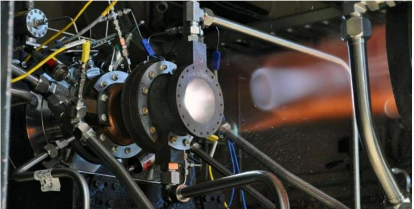
Aerojet Rocketdyne (AR) at NASA's Glenn Research Centre in partnership with NASA successfully completed the first hot-fire tests on an advanced rocket engine thrust chamber assembly using copper alloy materials.
