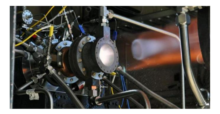
Aerojet Rocketdyne (AR) at NASA's Glenn Research Centre in partnership with NASA successfully completed the first hot-fire tests on an advanced rocket engine thrust chamber assembly using copper alloy materials.
